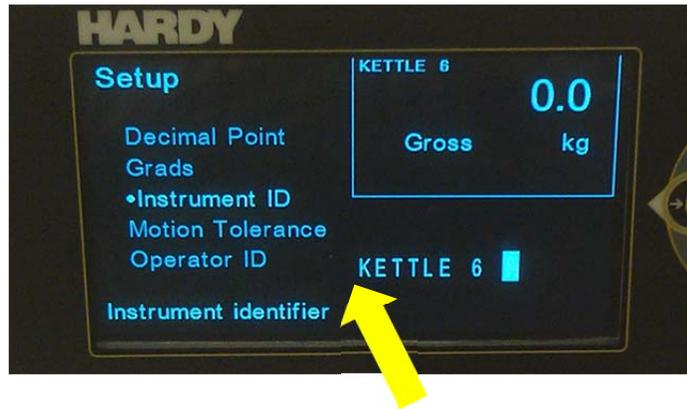
Press the enter key to save the customized instrument ID, then use the left arrow to back out of the set-up menu until the full screen mode is shown. As described above, toggle to split screen mode by pressing the enter key. Repeat as necessary for additional channels.
